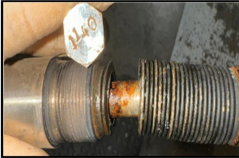
Fig.5: Gas Lift Valve Number Busted Bellow
